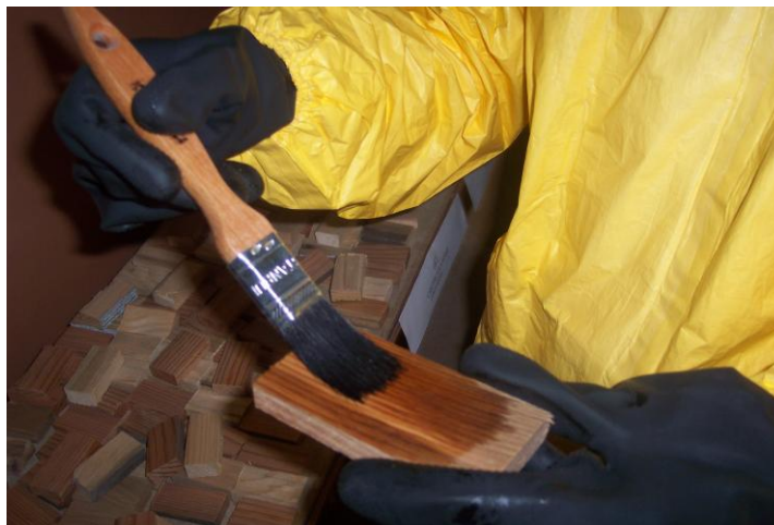
Figure 2.1. Applying treatment material via brushing method
